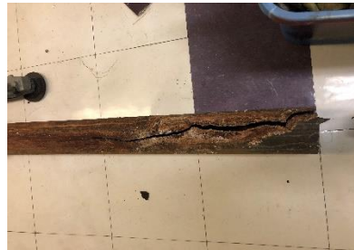
Image 1.3 This pipe was removed after a maintenance descaling and flushing of the main sewer and water
